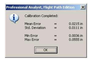
If the calibration statistics are unsatisfactory, you must check your sources of error. Check that all points have been located properly. Check that there is no unwanted distortion introduced by the camera lenses, mirror, or other optics.
