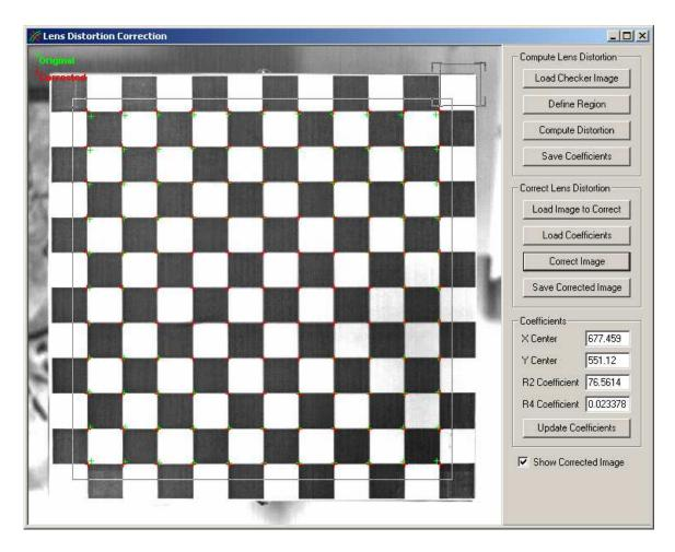
The **Correct Lens Distortion** options are provided only for verification of removal of distortion and as a tool for recovering undistorted images. These options can be used to correct other images and save the corrected versions if desired. This is not necessary since the application will automatically correct images on-the-fly if lens distortion coefficients are set.
