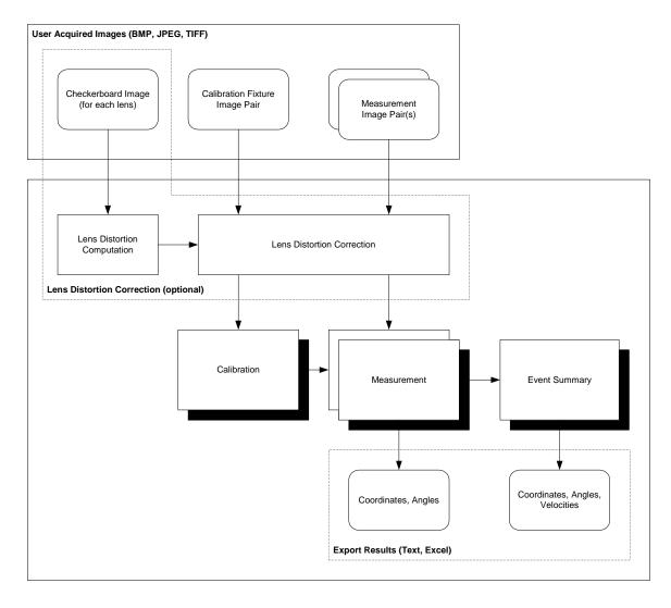
In addition to the Calibration and Measurement images, an optional Lens Distortion Correction tool is provided for removing radial lens distortion from images. If distortion is present in your lenses, then images of a checkerboard target should be taken using each lens and the resulting lens distortion correction computed. See the Appendix for more details on Lens Distortion Correction.
