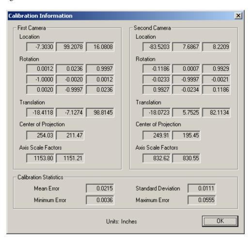
After the cameras have been calibrated, for every point that you click on in the top image, an epipolar line will be drawn in the bottom image and vice versa. The epipolar line
