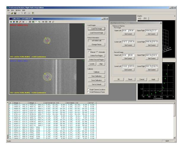
After all eight reference markers have been located, hit **Apply**. The location of these markers will be saved with the calibration information when the calibration is saved. These values will be using during measurement to try to compensate for any movement of the cameras between shots.
